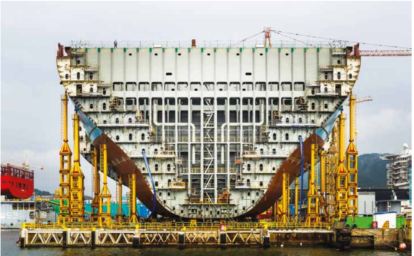
Triple E ship under construction in South Korea. These 400 metre-long ships with a capacity for 18,000 containers, are unable to pass through the Panama Canal. A Nicaraguan canal would cut 5,000-7,000 miles off journeys from Asia to the US eastern seaboard, the Caribbean and Latin America. Fewer ships, shorter journeys and greater fuel efficiency would mean a 35% reductions in CO 2 emissions, proponents claim
