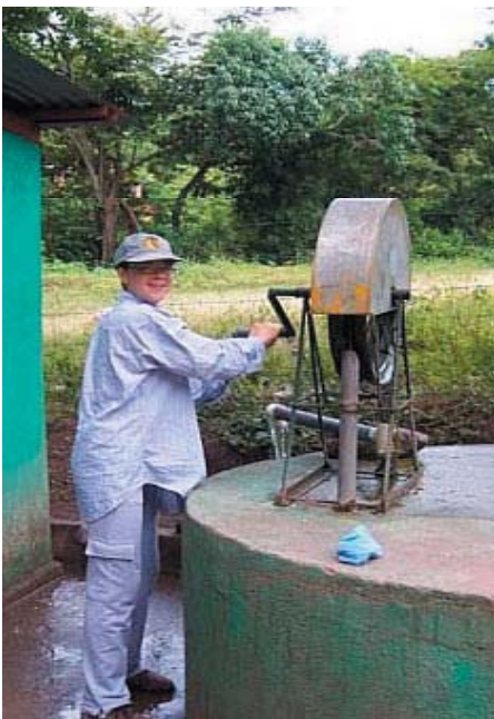
Volunteer from 2005 brigade demonstrates cistern for capturing rain water. Photo Laura Jensen
